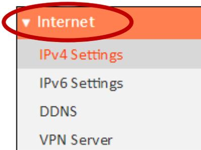
The “Internet” menu provides access to WAN IPv4, WAN IPv6, DDNS and VPN server settings. Click on an item from the submenu to view and/or configure the settings.
