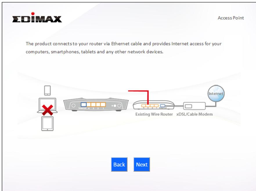
2. Connect the network port of your RG21S/RA21S to the LAN port of your existing router using an Ethernet cable, then click “Next”.
